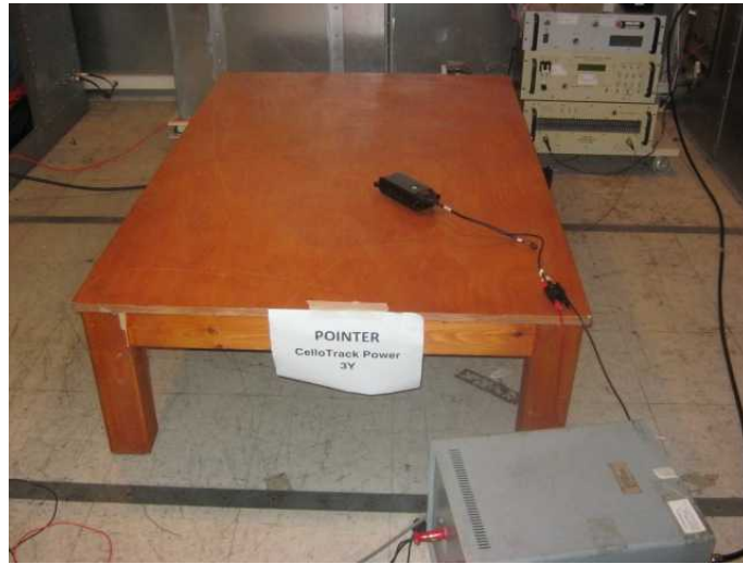
Figure 11. Conducted Emission From DC Port Test
